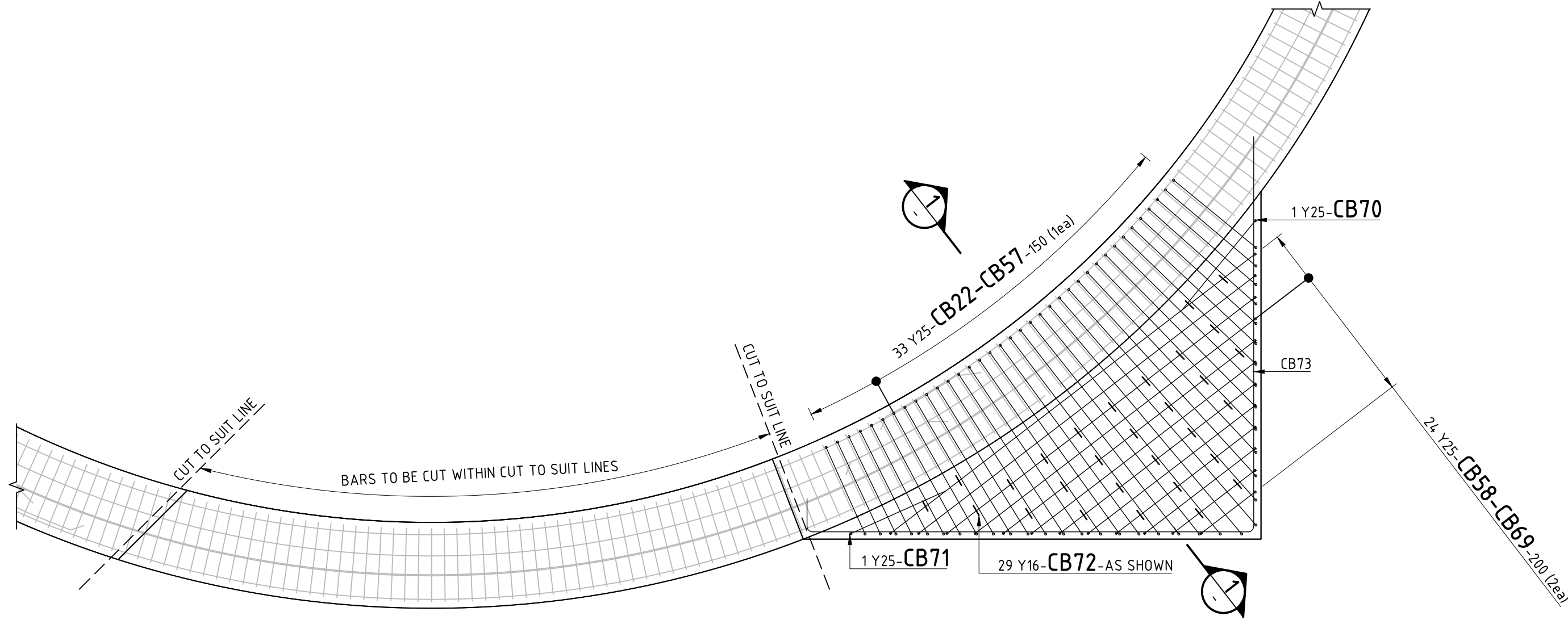
PART PLAN ON CAPPING BEAM STUB AND RECESS
